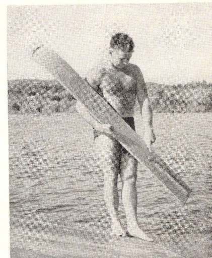
Sonny Cantin points to the pitot tube set forward of the skeg on the ski bottom.
